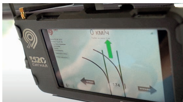
Onboard control and monitoring module with a touch screen
