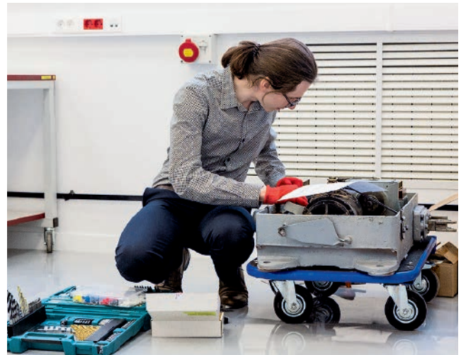
Testing of a point machine
