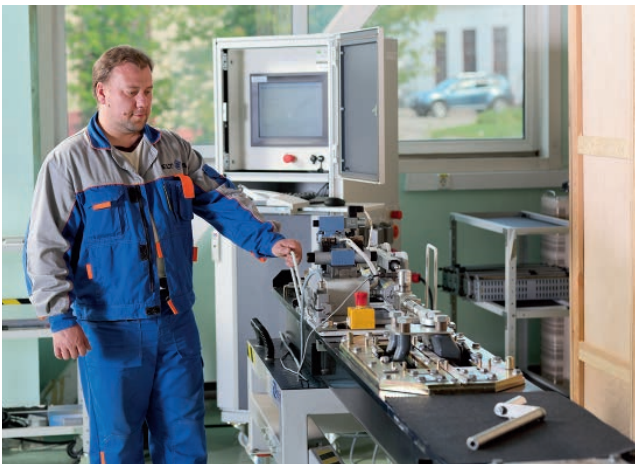
Laboratory testing of an in-sleeper electric point machine
