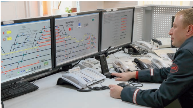
Mnemonic scheme of the Ugreshskaya station of the Moscow Central Ring (MCC) in the MultiRcos system
