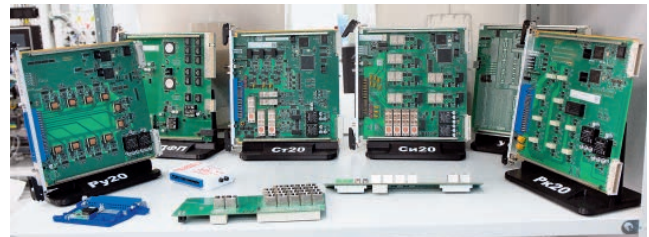
Cards of the PNU20 lower-level platform
