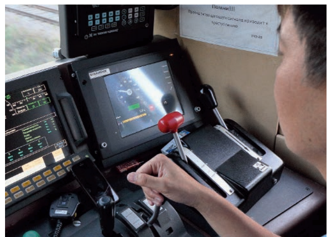
Display of the RBTC onboard safety system on the train operator's console
